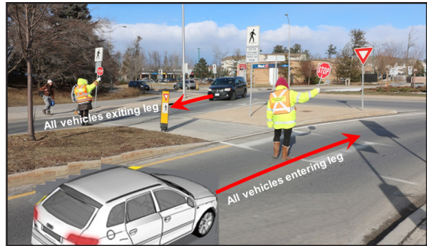
Figure 12-1 Conflicting Vehicular Movements at a Leg of a Roundabout
